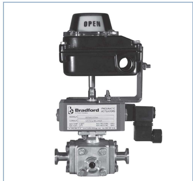
Dixon automated 1/2" 3-way 'L'-port encapsulated hygienic ball valve with double acting actuator and NEMA 4 limit switch with two SPDT mechanical switches and NEMA 4 115 VAC solenoid pictured. BV3SVLF050CBXC .
