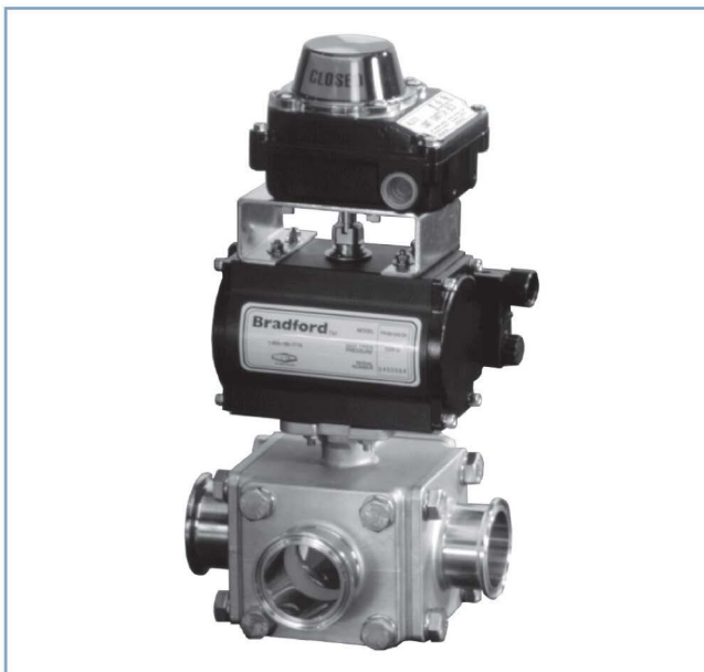
Dixon automated 1 1/2" 3-way 'L'-port encapsulated hygienic ball valve with double acting actuator and NEMA 4 limit switch with two SPDT mechanical switches and NEMA 4 115 VAC solenoid pictured. BV3SVLF150CBXC .
